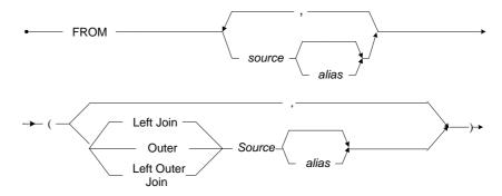
Figure 3-125 DBMaker Outer-Join Syntax
