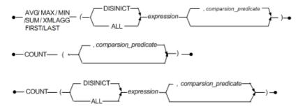
Figure 3-136 AGGREGATE FUNCTION syntax
