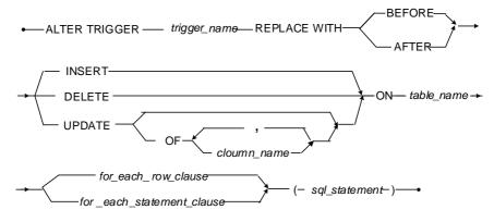
Figure 3-32 ALTER TRIGGER REPLACE syntax
